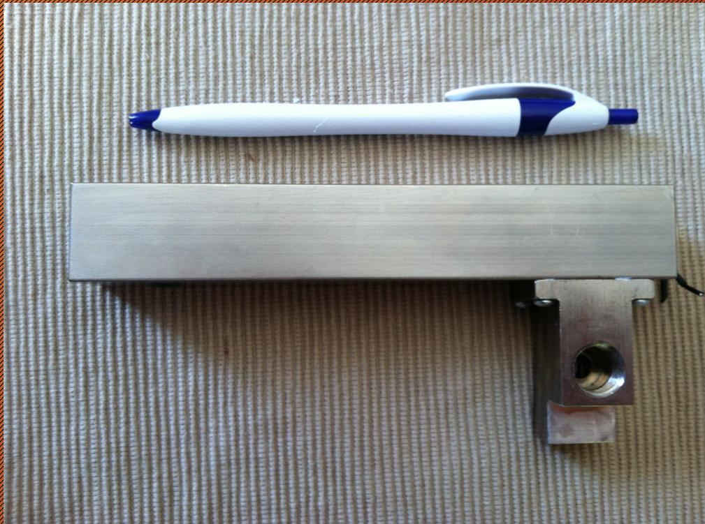
**Example of EC/IR Infrared chamber**
