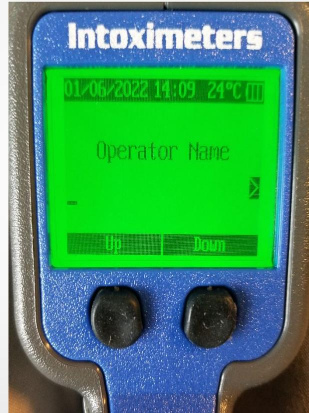
The first screen will be Operator Name and you will transition to the keyboard for data entry after ASV is in its docking station/cradle.
